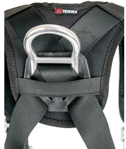
This single attachment point harness is extra light and extra comfortable. D-ring and connecting buckles are made from aluminum alloy. Each buckle connection unit has an additional (extra) male buckle to secure the slack end of webbing. Such construction helps to avoid any slippage of a webbing for highest safety.
