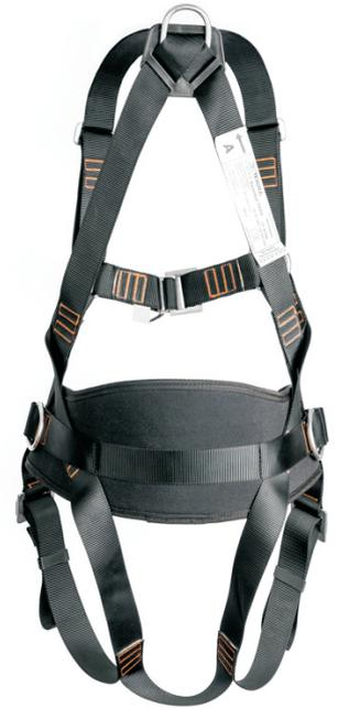
This 4-point harness combines simple and ergonomic harness with comfortable work positioning belt, two-in-one. The harness is fitted with a rear D-ring and two side D-rings mounted to the belt for pole climbing or can also be used for work positioning on various open structures. It also has a front D-ring attachment point.
