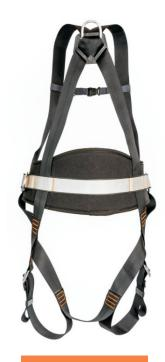
This 3-point harness combines simple and ergonomic harness with comfortable work positioning belt, two-in-one. The harness id fitted with a rear D-ring and two side D-rings mounted to the belt for pole climbing or can also be used for work positioning on various open structures.
