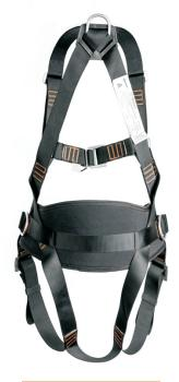
This 4-point harness combines simple and ergonomic harness with comfortable work positioning belt, two-inone. The harness id fitted with a rear D-ring and two side D-rings mounted to the belt for pole climbing or can also be used for work positioning on various open structures. It also has Frond D-ring attachment point.
